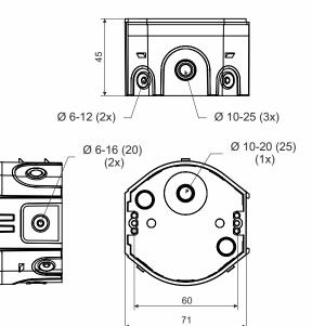
product description: designed for distribution system with voltage 400 V and with maximum current 16 A
