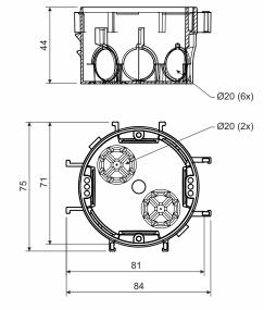
product description: designed for distribution system with voltage 400 V and with maximum current 16 A for modern installations in combined frames vertical and horizontal connection with a spacing of 71 or 81 mm (up to 5 boxes) possibility to increase axial distance with a spacer for the design lines Element, Neo allows to install double-socket
